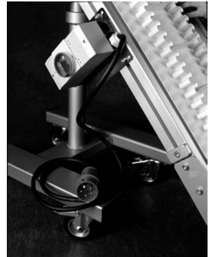
Figure 3-5: Motor overload switch
